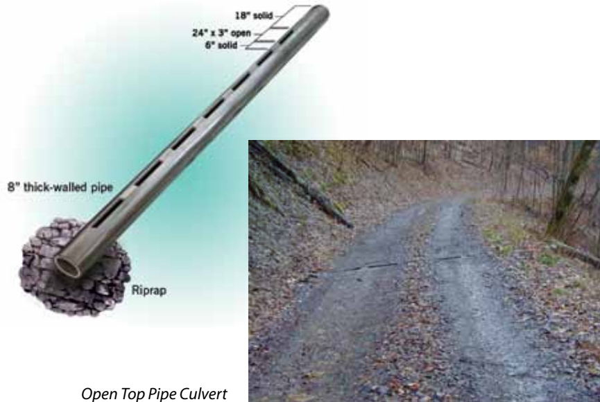
Open Top Pipe Culvert
